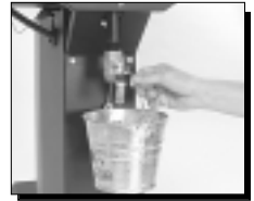
Drain Valve & Bucket
